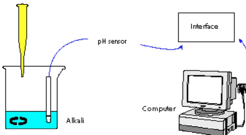
As acid drains into alkali the pH changes. This can be monitored using a pH sensor and instantly produce a graph of pH against volume. The volume of acid added is entered using the keyboard. The experiment can be repeated using different combinations of strong and weak acid.
