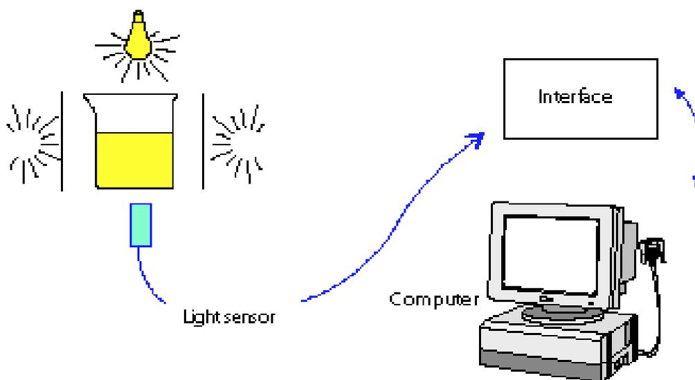
Sodium thiosulphate and acid react to form a precipitate. The light sensor can be used, like a colorimeter, to monitor the rate of the reaction. In this experiment we study the effect of different amounts of acid on the reaction rate. It will also be possible to study the effect of temperature.
